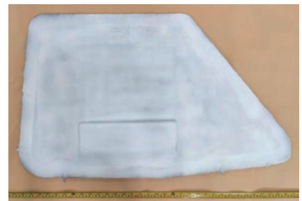
图 10 四层板舵翼成形结果 Fig.10 Experiment result of four-sheet rudder wing
